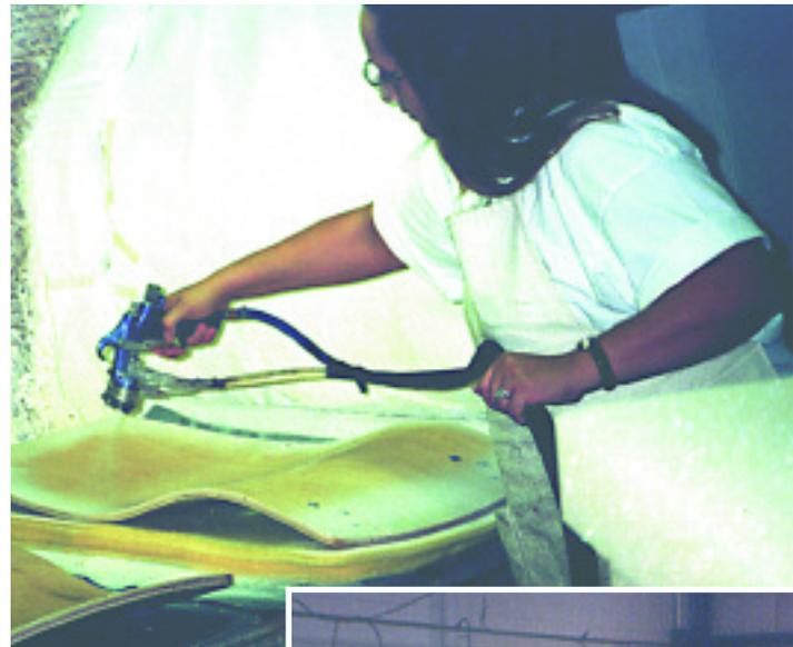
*Instant bonding and excellent green strength is provided here to maintain contact of the foam to the wood in this waterfall edge seating application.*
